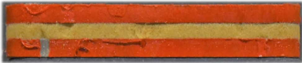
40/70 White With FR Between Two Steel Cores
